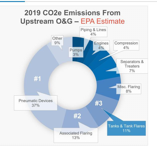
Based on the latest EPA Greenhouse Gas Inventory, pneumatic devices represent the largest source of CO2e emissions, followed by Associated Gas flaring, then tanks and tank flares.
